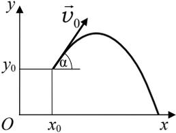
$\begin{cases} x(t) = x_0 + v_{0x}t = x_0 + v_0 \cos \alpha \cdot t \\ y(t) = y_0 + v_{0y}t + \frac{g_y t^2}{2} = y_0 + v_0 \sin \alpha \cdot t - \frac{gt^2}{2} \end{cases}$ $\begin{cases} v_x(t) = v_{0x} = v_0 \cos \alpha \\ v_y(t) = v_{0y} + g_y t = v_0 \sin \alpha - gt \end{cases}$ $\begin{cases} g_x = 0 \\ g_y = -g = \text{const} \end{cases}$ |
